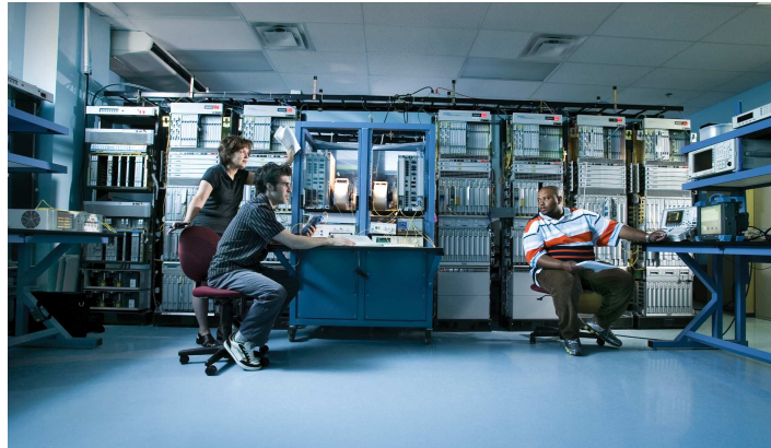
Optical Recirculating Loop Test Bed based on Nortel 10G WDM Transmission System Laboratoire de technologies de réseaux Christine TREMBLAY resp.
